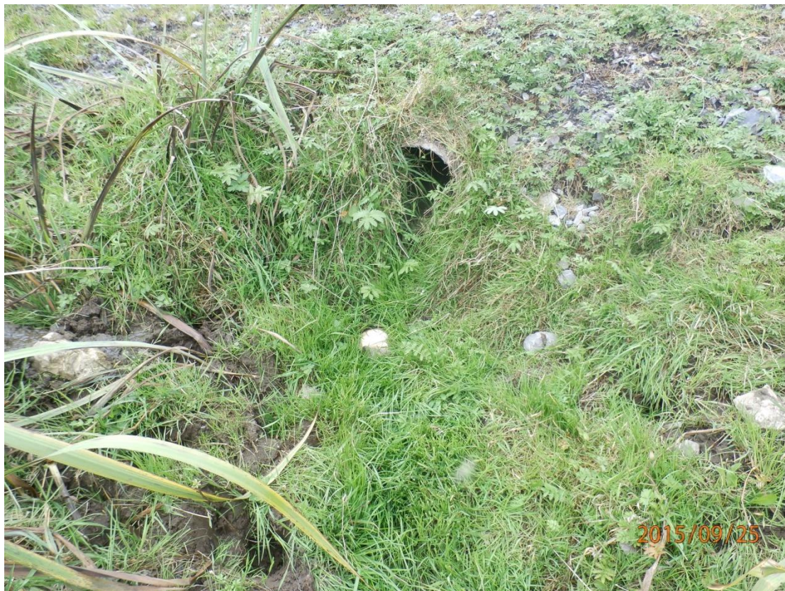
Underpass Cotton Wool sample collected to establish groundwater flow from Swallow Hole No 2 Collecting: 25/09/2015
