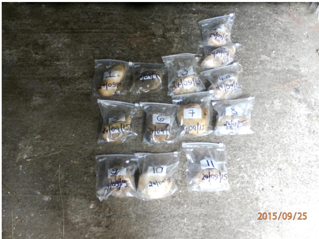
Cottons 1 - 11 collected on 25 th September 2015 Cotton Wool sample collected to establish groundwater flow from Swallow Hole No 2
