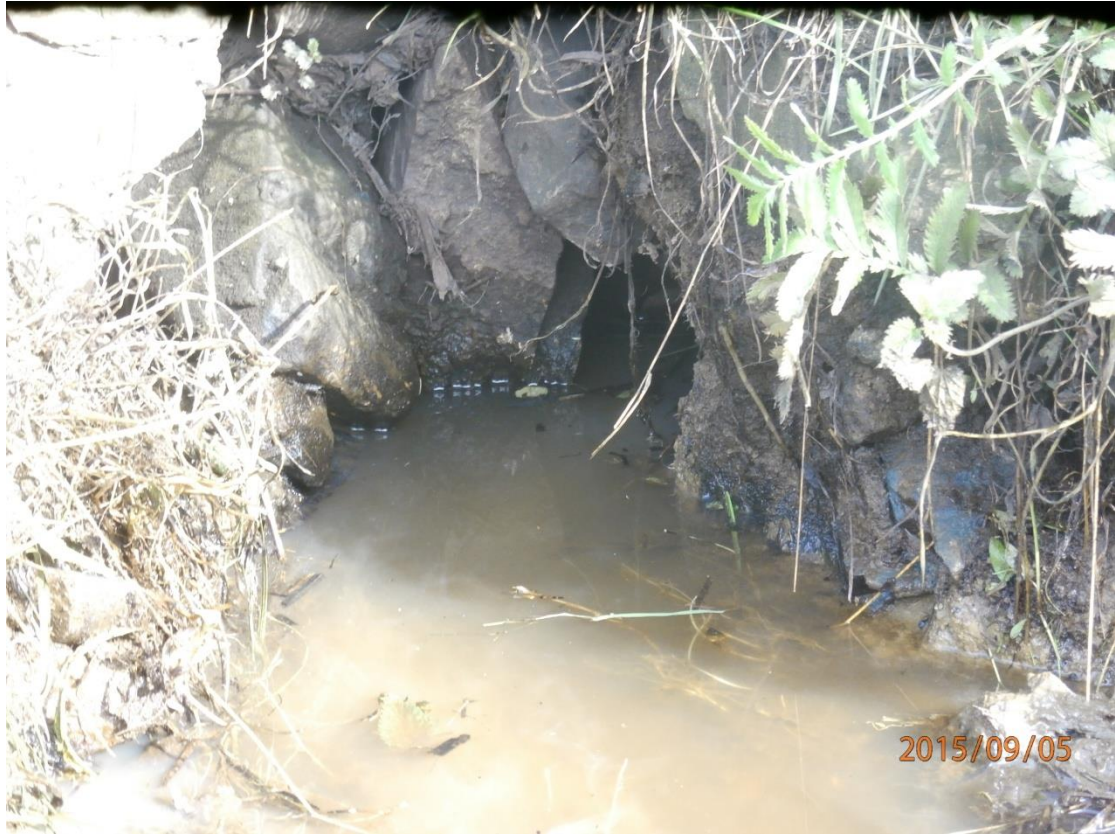
Swallow Hole No 2 at Sheep Field 12.5 litres of ultrabrite poured in Swallow Hole No 2 at 16:00 hours on Saturday 05 th September 2015
